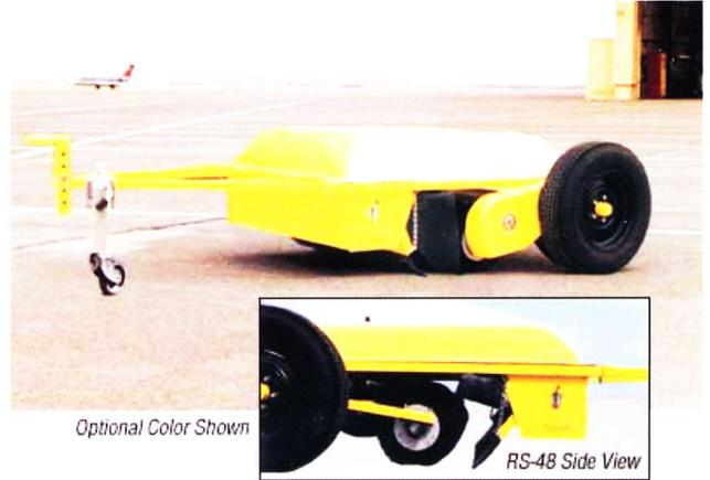
Your FOD removal costs will drop dramatically once you hook up one of these efficient, traction-driven units to your flightline vehicles turning them into powerful sweeping machines. All motors, hydraulic, vacuum attachments, and fuel have been eliminated as well as the man-hours, parts and downtime required to repair them.
